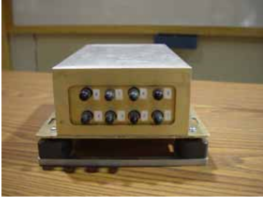
Figure 1a. Photograph of flight qualified 8-channel AEROSCAN optical fiber sensor support system
