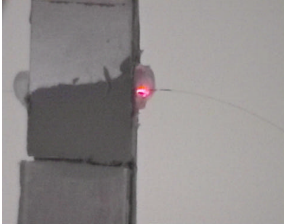
Figure 15. Checking integrity of grating sensor with visible light source after joint failure.
