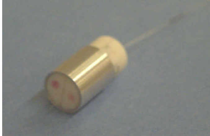
Figure 1. A partially completed assembly of the corrosion sensor developed by the authors (Actual prototype size: 0.4" L x .25" Dia).
