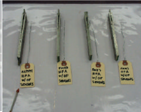
Figure 10. Photograph of the various wedge samples with embedded optical fiber Bragg sensors after 100 % RH / 140 °F exposure for 24 hrs.
