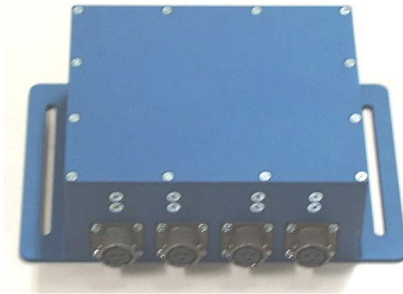
Figure 4. Battery Operated Health Monitoring System Unit Battery Pack.
