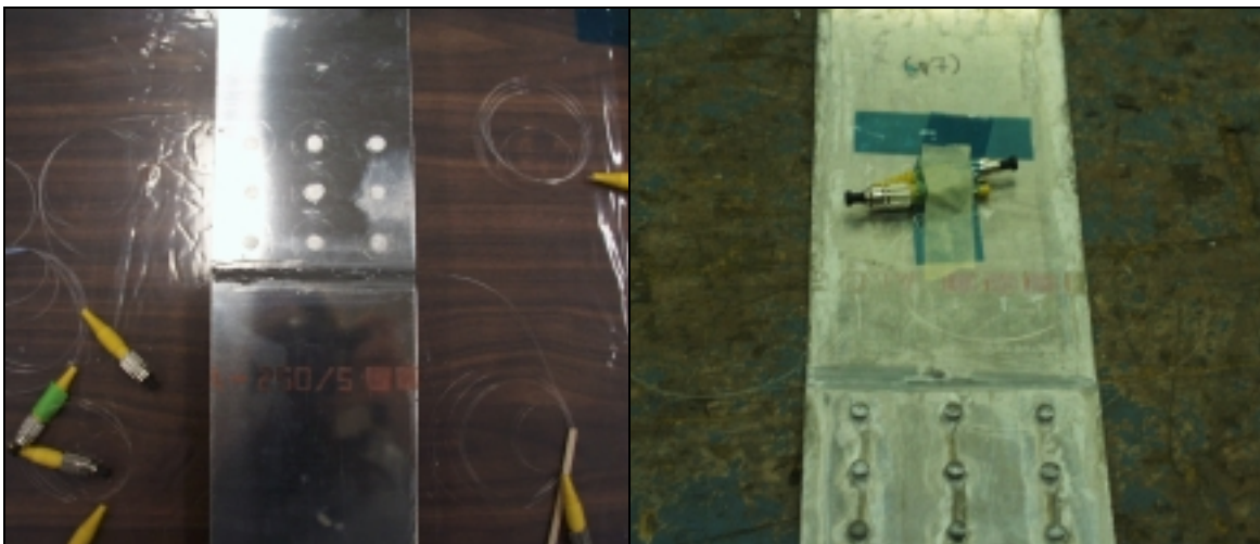
Figure 7a. Photograph of simulated lapjoint with embedded long period grating-based moisture sensors in lapjoint crevice under aircraft sealant.
